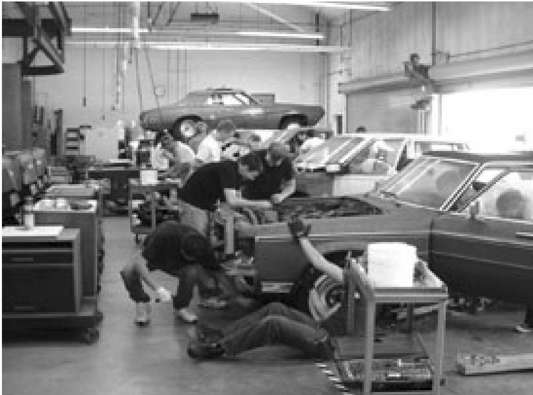
Preparing to pull an engine, AUTO 104B — Automotive Engines
