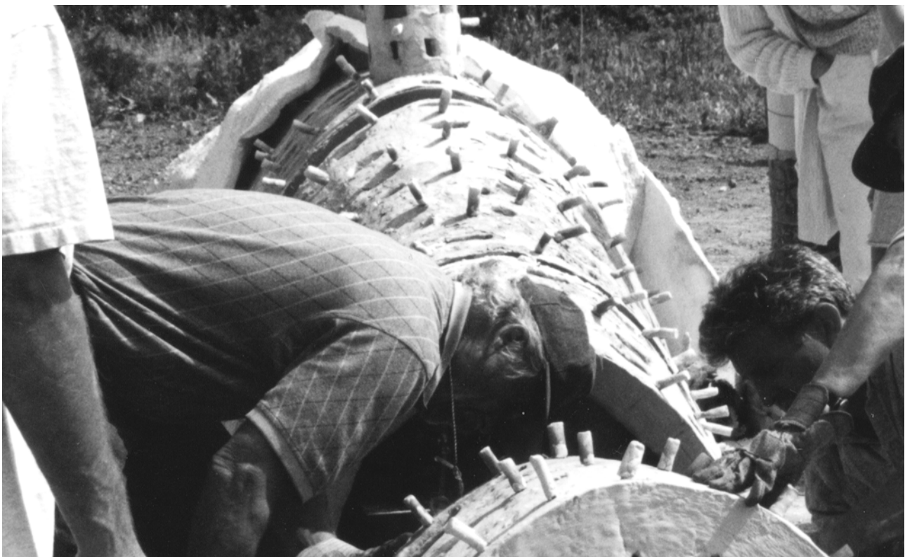
The kiln was covered with a refractory blanket and slowly heated to 2300 degrees Fahrenheit over the course of several days.
