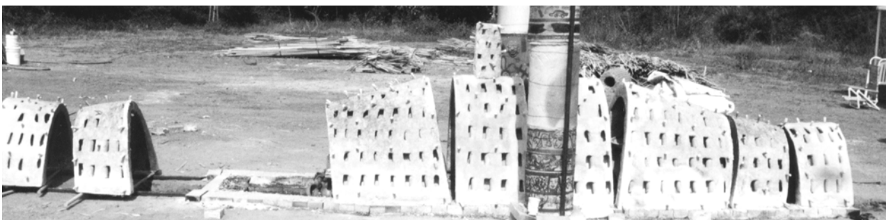
The 14-foot-long, 4-foot-high, 3-foot-deep kiln was handbuilt from a coarse clay material.
